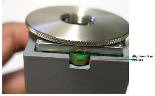
4) Gently push the Filament Film NeuroPort plug onto the head stage housing of the Patient Cable. Do not touch the filament film or the alignment pins inside the plug.
