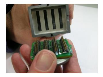
3) Take the beta sample of the Filament Film NeuroPort plug and lay it on the head stage housing of the Patient Cable such that key feature of the Filament Film NeuroPort plug aligns through the slot on the housing of the head stage as shown in the figure below.
