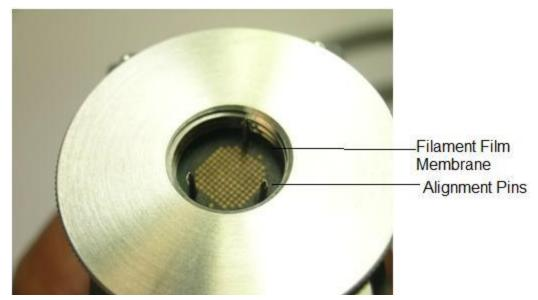
5) Make sure the black conductive rods on the sides of the head stage housing are touching the flanges of the Filament Film NeuroPort plug as shown in the figure below.
