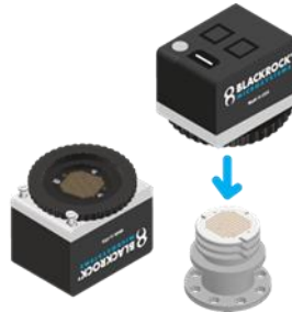
Figure 4 —Proper orientation of the CerePlex E relative to the CerePort Pedestal. Note how the notches in the Pedestal align with the guide pins in the CerePlex E when
