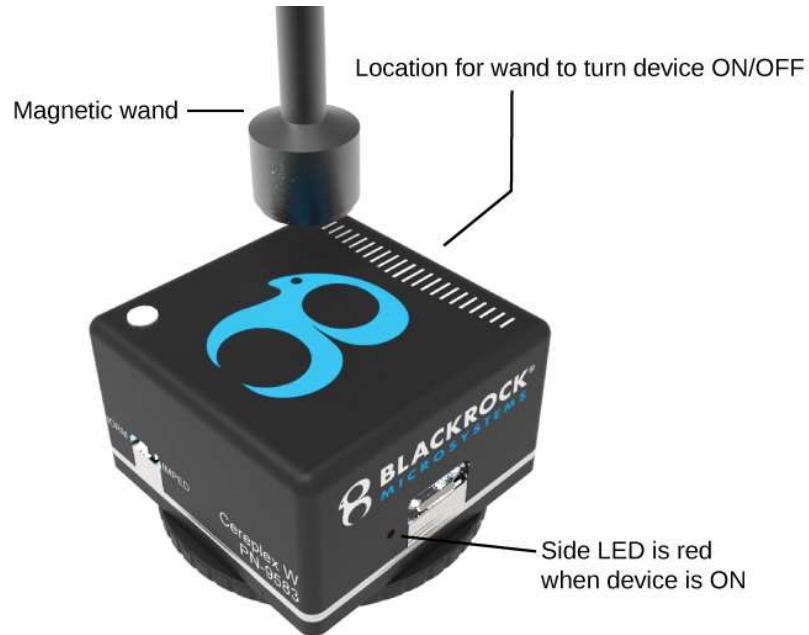
Figure 2—Turning on the power of the CerePlex W headstage using the magnetic wand.
