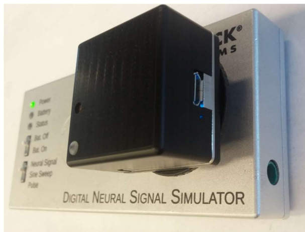
Figure 11—The CerePlex W headstage connected to the pedestal connector of the DNSS.
