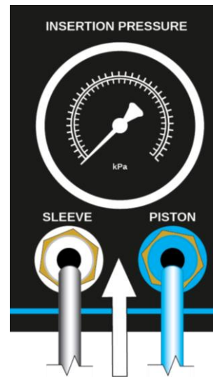
Figure 6: Close-up of tube placement on inserter
