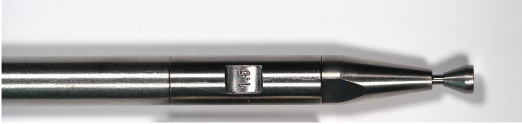
Figure 7: Close-up of wand spacer. Spacer length in mm is engraved on the spacer. 1.5 mm
